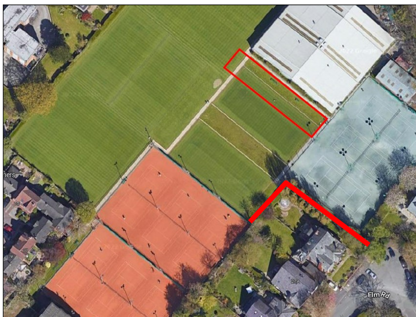
Proposed location of the padel courts outlined above, with the single red line indicating the approximate position of the proposed acoustic fence to the Elm Road boundary
